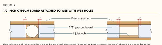
This solution only requires the web to be covered. Fasteners (Type W or Type S screws or nails) should be 1 inch from the edge and end of the gypsum. Gypsum is not required above or below openings, no matter what the opening size is. Round, square and rectangular web holes are permitted, provided the requirements for hole placement and size meet the 1-joist manufacturer's APA Product Report or code evaluation report.
